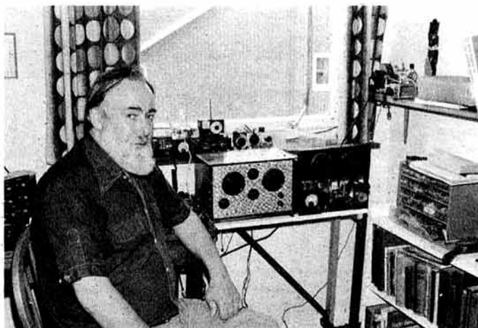
Richard Farley, GW3SSJ, with his re-constructed "1920s" equipment. The "Empire Two" receiver on the right uses 2V battery valves, it, gb and ht batteries etc, with engine-tuned front metal panel. The single-valve transmitter was built about 25 years ago using an LS5A as specified in 1927 but now usually uses a 415PT valve dating from 1928 (4V directly-heated pentode) that runs at about 7W input. As a self-excited oscillator on 7MHz GW3SSJ got T7C reports but as a usable co gets good T9 reports from around Europe. The LS5A (but not the 415PT) gives enough light to operate by!
